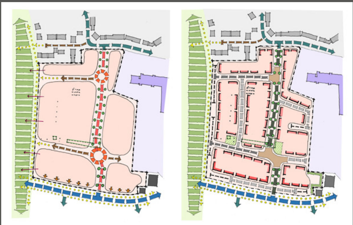
Concept and development framework plans for the residential development at Llanwern show how the analysis has been interpreted and developed to give the site structure. (Image courtesy of Roberts Limbrick)
